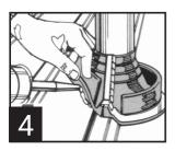
Press the Dektite base to contour of roof profile.
