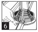
Apply sealant to top of crimp closure and any other potential leak areas.
