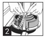
With clip in down-stream position, tension top of cone around pipe and engage metal teeth in opposing pockets.
