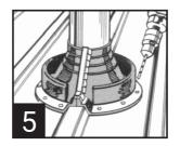
Fasten flashing with washered self drilling screws.
